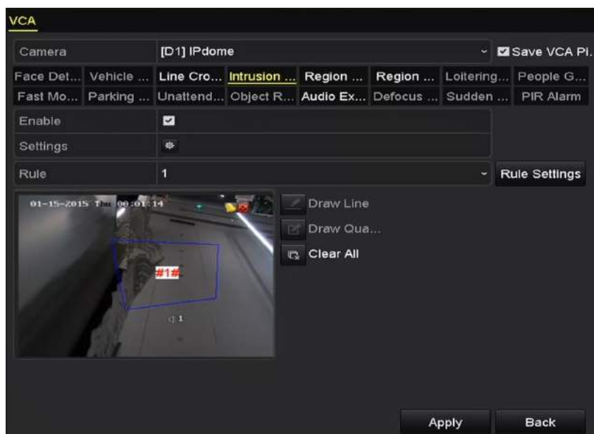
Figure 10-8 Draw Area for Intrusion Detection
