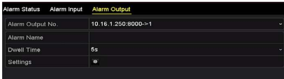
Figure 8-19 Alarm Output Settings Interface
