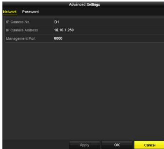
Figure 2-29 Network Configuration of the Camera
