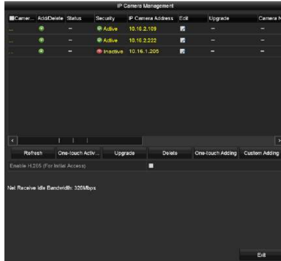
Figure 2-21 IP Camera Management Interface
